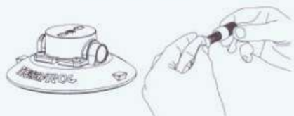
Clean the inside of the cylinder and the plunger with a lightly wet paper towel
