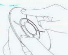
Check to ensure there is no scratch on the edge of the vacuum cup.
