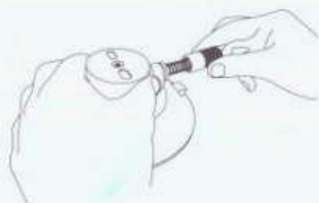
Pull the plunger straight out from the pump cylinder.
