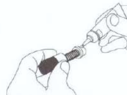
Re-lube the rubber O-ring with a thin layer of silicone gel
