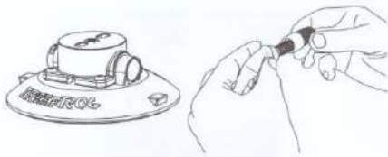
Clean the inside of the cylinder and the plunger with a lightly wet paper towel
