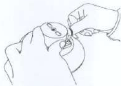
Push the plunger back into the cylinder and pump several times to ensure the pump move back and forth freely and smoothly
