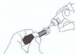
Re-lube the rubber O-ring with a thin layer of silicone gel
